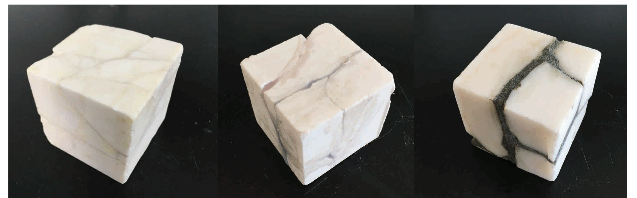
Microbial repair, epoxy repair, and cement repair of broken white marble blocks (from left to right)
