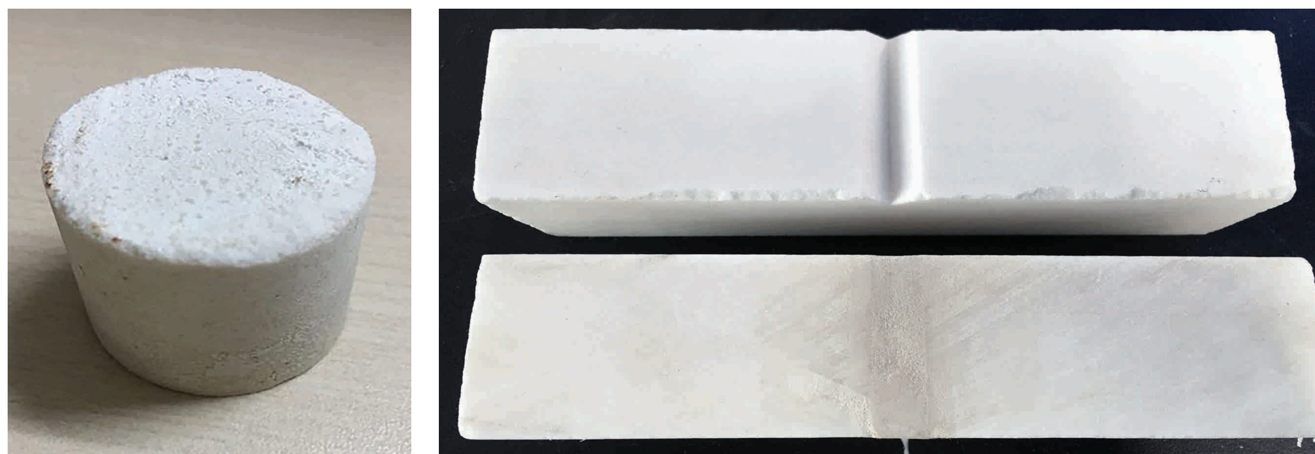
High strength (55MPa) microbial induced sandstone (left panel); Groove-filled white marble stone before (upper right panel) and after repair (bottom right panel)
