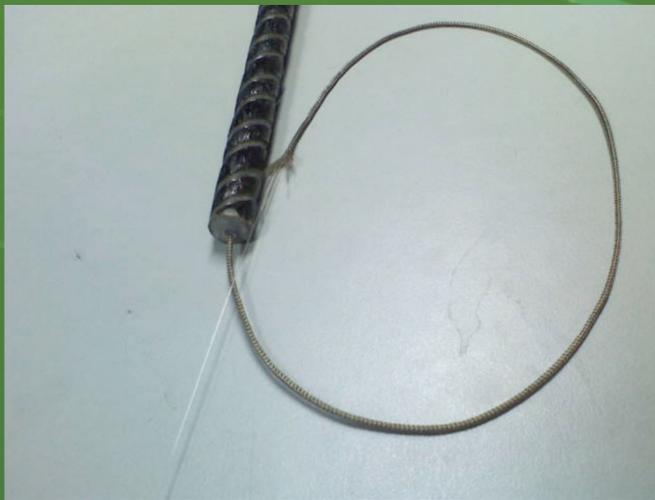
*Smart Basalt Fibre Reinforced Polymer*
