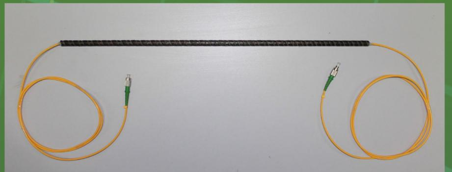
*Smart Basalt Fibre Reinforced Polymer*
