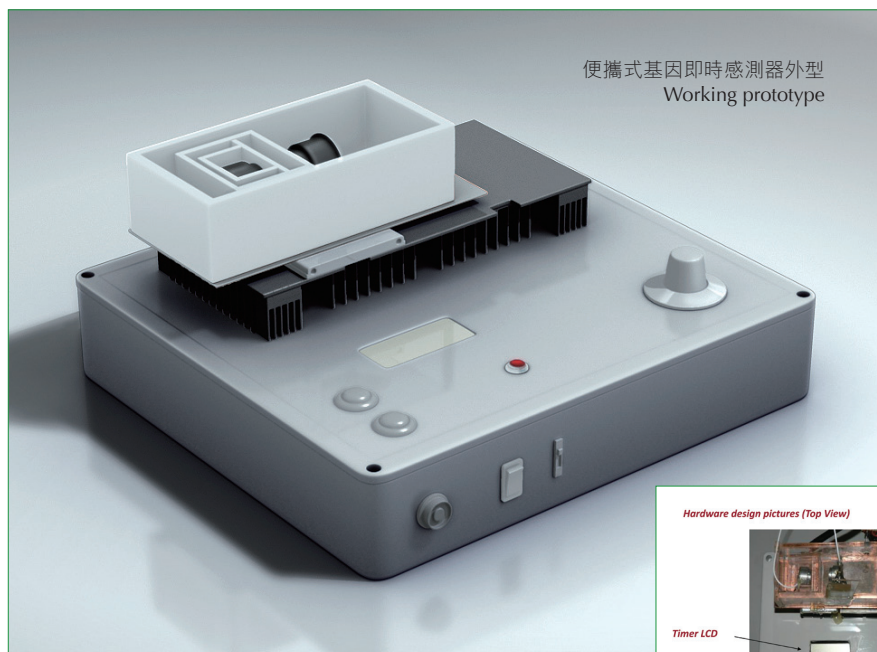
便攜式基因即時感測器包括了測試樣本培植槽和凝塊自動檢測裝置 This hardware provides an incubation environment and auto-detection of clotting
