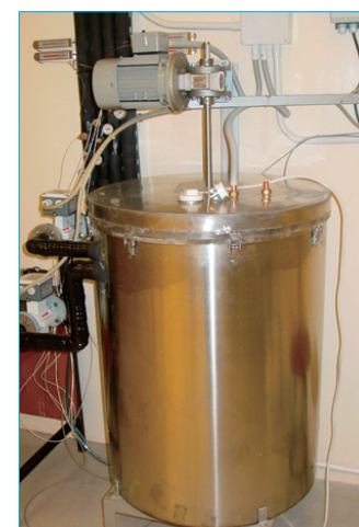
示範裝置：夜間電蓄冷微膠囊相變材料蓄能裝置 Prototype: MPCM slurry storage of night time electric cooling
