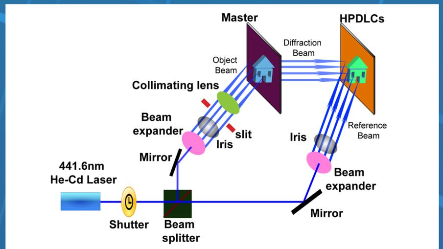
(Fig. 2) Setup for holography
