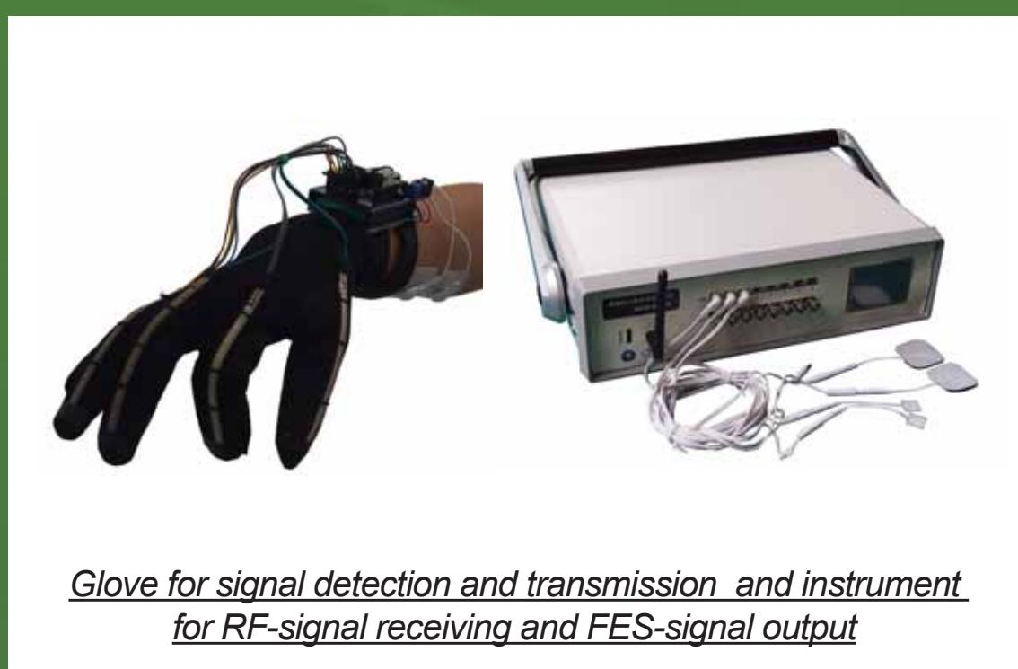
Glove for signal detection and transmission, and instrument for RF-signal receiving and FES-signal output
